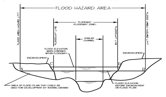
LINE A-B IS THE FLOOD ELEVATION BEFORE ENCROACHMENT LINE C-D IS THE FLOOD ELEVATION AFTER ENCROACHMENT
